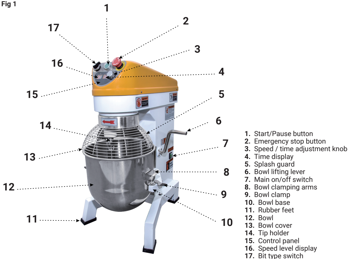
Figure 1 Construction of the device
